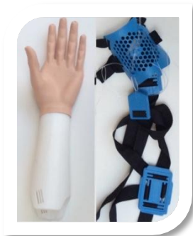
Final 3D printed LifeArm
